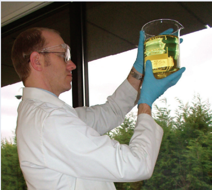
A technician carrying out a 'clear and bright' analysis of a fuel sample. An extremely subjective method due to the fact that the human eye can only see down to 40 microns unaided.
