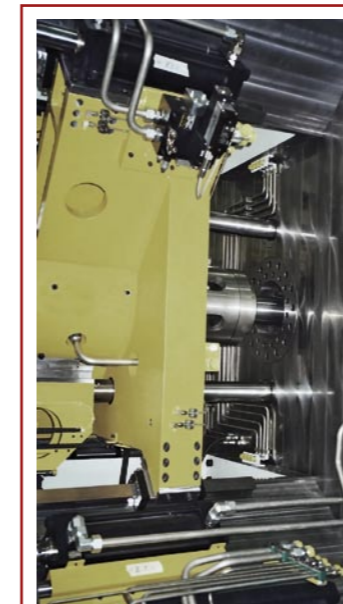
Metal spinning and flowforming machines used to manufacture wheel rims must generate enormous forming forces in order to shape even when the materials are thick. This process involves the thinning of material in specified regions, generating the desired rim shape.
