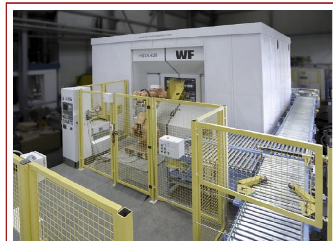
For heavy-duty metal spinning and flowforming processes, WF Maschinenbau offers horizontal implementations, such as the Type HSTA625 machine. In these machines, the rotating working spindles and tools are pushed along the axis of the machine through the fixed support along with the radial feed units.
