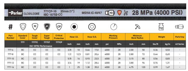
Reinforcement: Four-spiral steel wire
