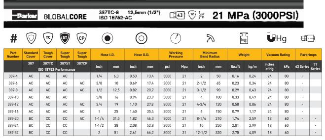
Reinforcement: One- or two-braid steel wire for sizes -4 to -16 | Four-spiral for sizes -20 to -32
