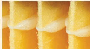
Adhesive beads bond the pleats into a rigid pack for even loading and complete media utilization.
