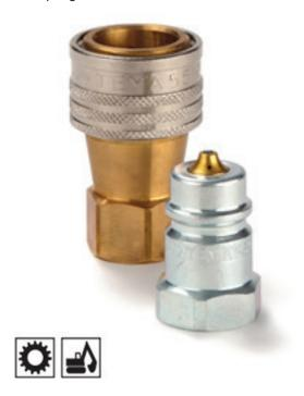
**RSD Series** is a one hand operated push-pull version, which serves to prevent leakage and destruction of the hydraulic hoses by automatic disconnection in case of accidental traction on the hose. The integrated detent system prevents circuit shut off in back-flow.
