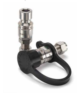
Parker FMS Series receptacles are designed for rigid mounting on a compressed natural gas vehicle. Receptacles can be employed in both fast-fill and time-fill dispensing applications. The ANSI/NGV1 standard used by FMS Series receptacles allows vehicle fueling to be accomplished with all CNG nozzles conforming to the ANSI/NGV1 standard.
