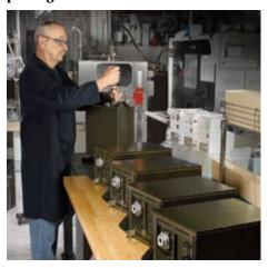
Ruggedized enclosure and liquid flowthru board, line replaceable modules (LRMs) compatible with VITA 48.3, IEEE 1101.2 standards provide cooling of heat loads as high as **4000 W for a 1-ATR chassis** (approximately 8" H x 10" W x 20" L) and board-level direct heat fluxes **as high as 25W/cm²** (thermal resistivity
