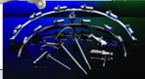
F414 nozzle with after- burner spray- bars and manifold
