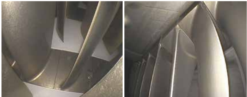
Fig. 1. Photos of 8000hr borescope inspection on an aeroderivative GT used for LNG processing - no water washing (Parker designed air intake).
