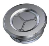
Reduced thickness in the membrane creates controlled rupture of the Parker Ship-N-Seal plug during final assembly
