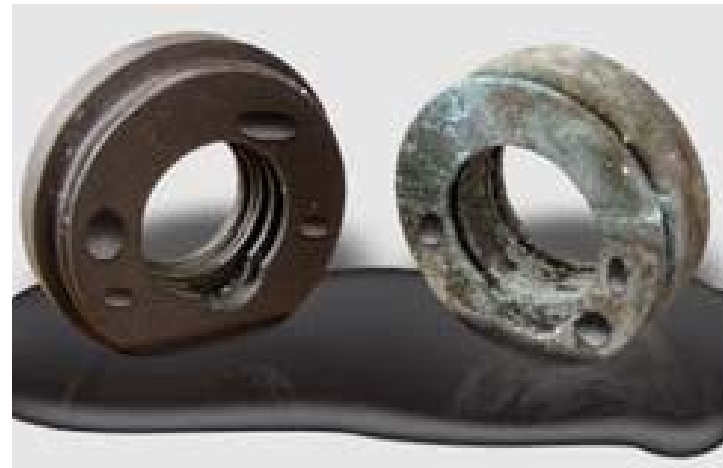
PTFE vs. metal after sulfuric acid soak
