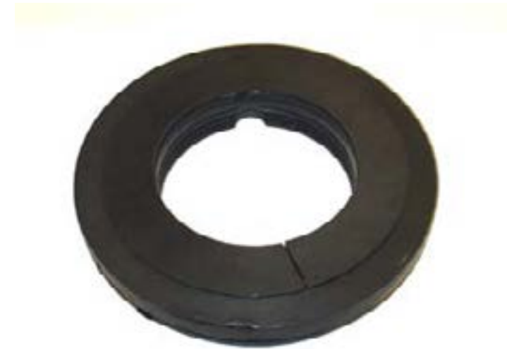
Failed seal resulting from improper fit
