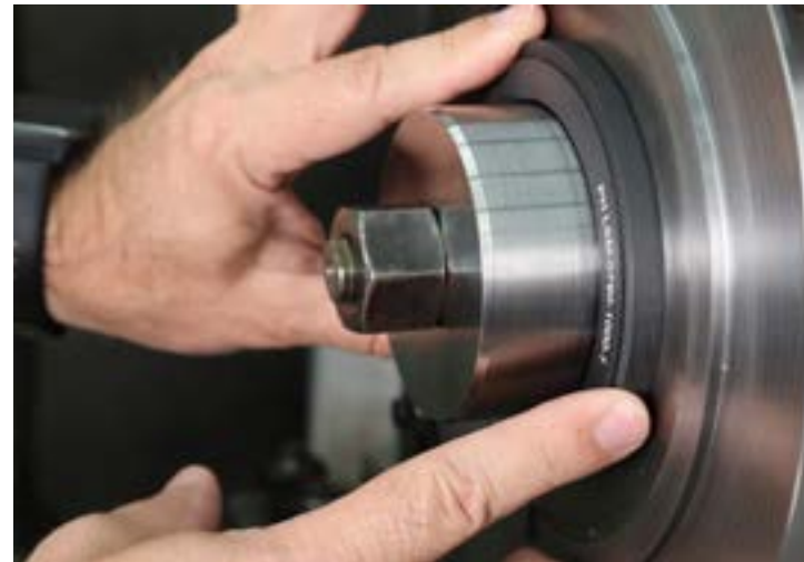
Installing the Seal
