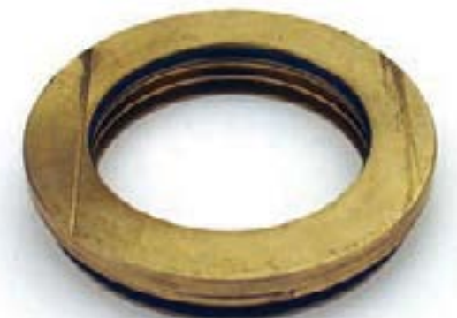
Failed seal resulting from improper installation
