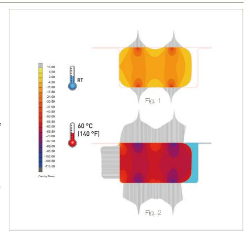
protection against twisting of the seal is achieved, both during installation and in operation at pulsating pressures, for instance in combination with breathing components and coaxiality defects of the groove. The use of particularly extrusion- resistant materials, especially Parker polyurethane compounds with 90
