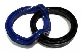
Polyurethanes are a thermoplastic elastomer. High heat causes the material to soften. Resilon 4350 seal (black) and Leading Competitor seal (blue)
