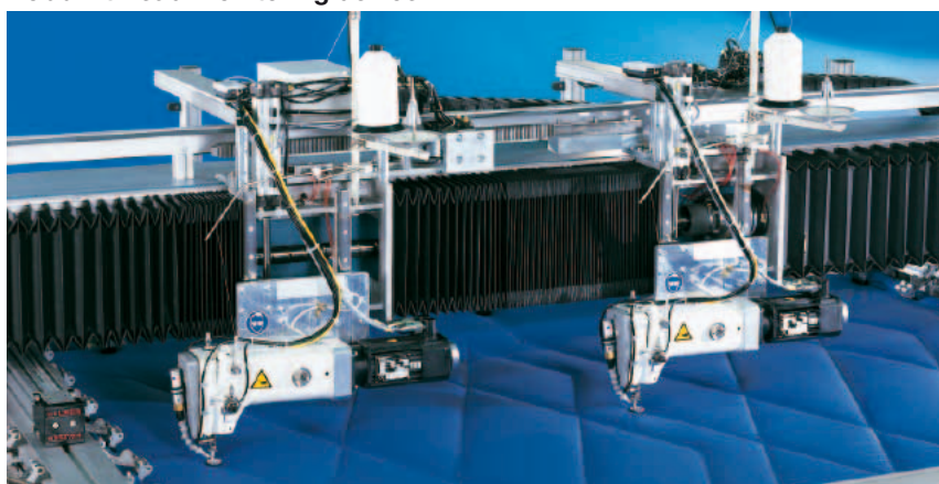
Quilting systems with double heads for increased efficiency
