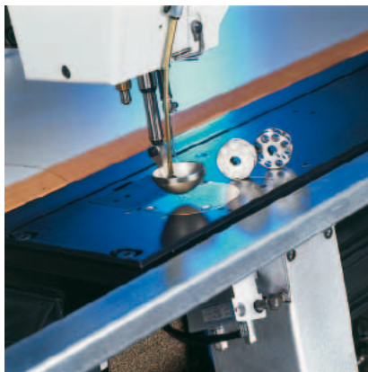
Large bobbin capacity with heavy-duty sewing head
