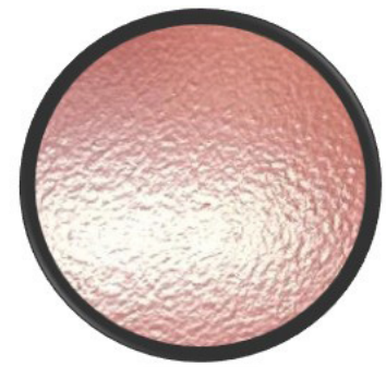
Surface Finish as applied via HVLP Gun
