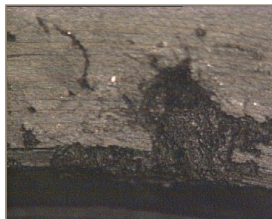
Pitting on filter end-cap
