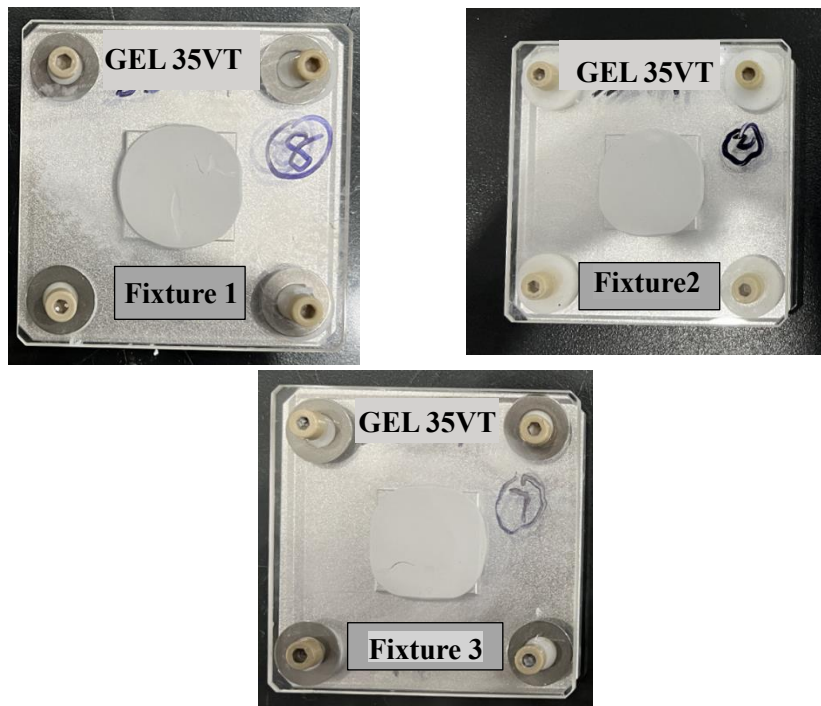
Figure 7: Automotive Testing Results after 3 Environmental Aging Tests
