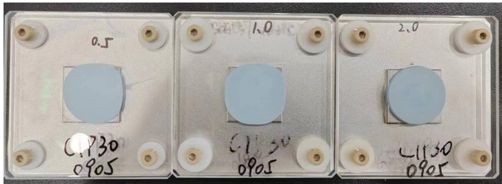
Specimens after thermal shock, temperature cycling and 2 types of vibration test
