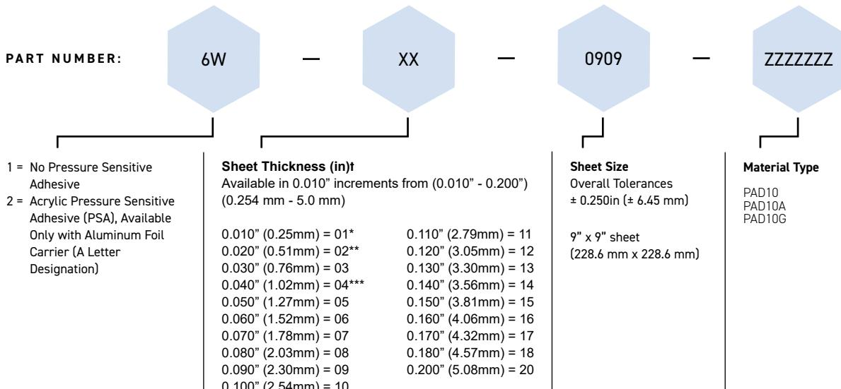
\* Minimum thickness for PAD10A is 0.010" (0.25mm)
