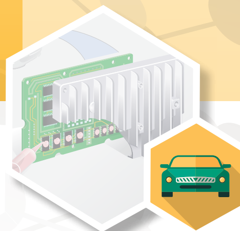
Dispensed Gels in Automotive Electronic Control Unit (ECU) Applications
