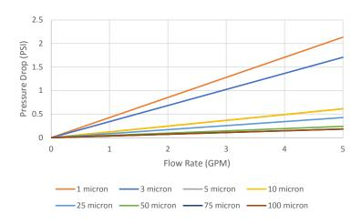
Flow rate is per 10" cartridge. For liquids other than water, multiply the pressure drop by the fluid viscosity in
