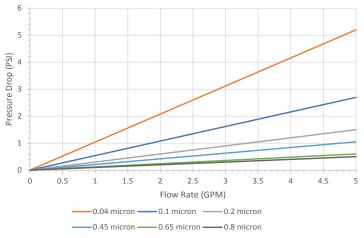
Flow rate is per 10" cartridge. For liquids other than water, multiply the pressure drop by the fluid viscosity in centipose.
