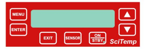
The front panel consists of a user interface, which includes an alphanumeric display and a membrane keypad to select operational modes and alarm settings. The display is a two line, 20 character, liquid crystal display (LCD). The display is backlit to allow easy viewing over a wide range of lighting conditions.
