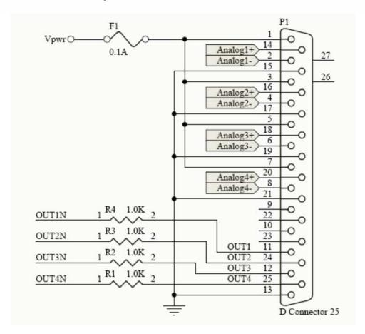
For 4-20 ma output of Conductivity (Analog 1), use pins 2 (4-20 -) and 14 (4-20 +). If excitation is needed in the loop, connect pin 1 (Vpwr) to pin 14 (4-20 +), and connect the output (signal) cable to pin 2 (4-20 -) and pin 15 (Gnd).
