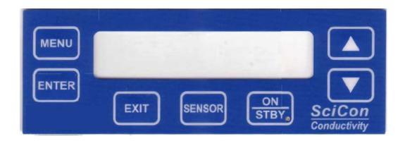
The front panel consists of a user interface, which includes an alphanumeric display and a membrane keypad to select operational modes and alarm settings. The display is a two line, 20 character, liquid crystal display (LCD). The display is backlit to allow easy viewing over a wide range of lighting conditions.
