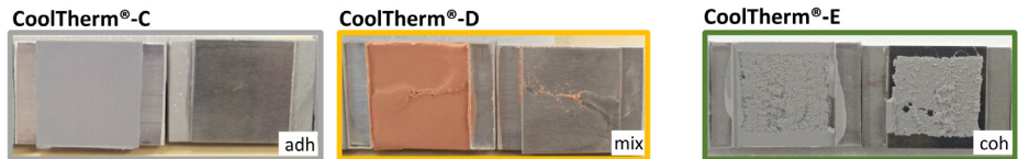
Figure 8. Comparing pull-off stress for Parker Lord gap fillers. The measurement was performed on aluminum surface with bondline thickness of 1 mm at pull-rate of 12 mm/min.
