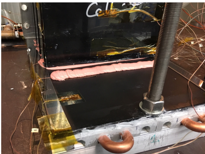
Figure 4: Assembly of battery cells onto cooling plate using a Parker LORD gap filler
