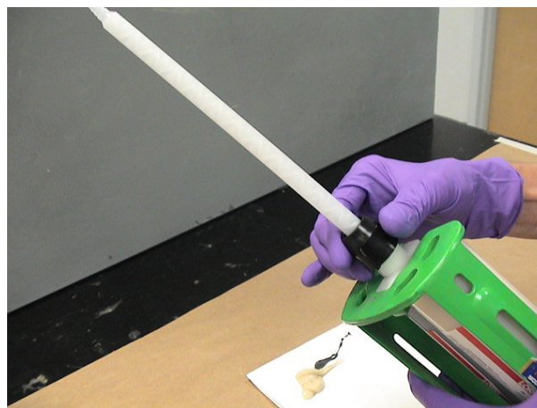
Attach static mix tip to cartridge
