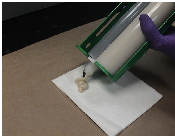
Level plungers in the cartridge
