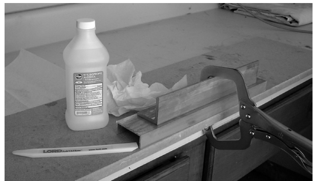
Rubbing alcohol removes smears or residue
