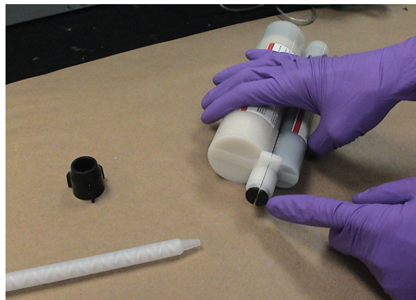
Remove and discard plastic plugs in outlet ports
