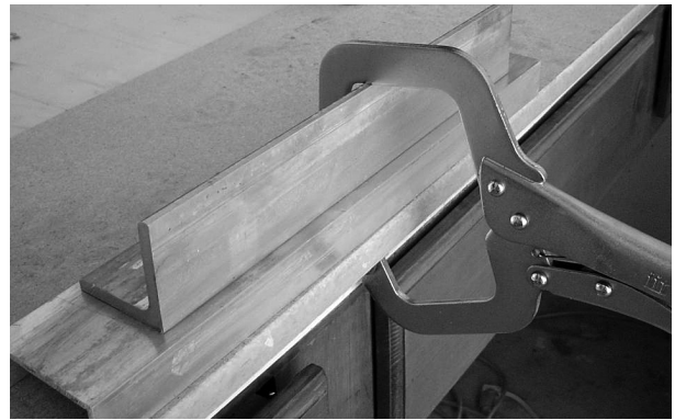
Clamp parts for required handling time
