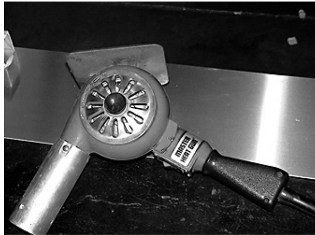
Use heat gun to remove bonded part
