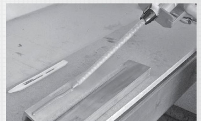
Figure 6 Position and dispense adhesive.
