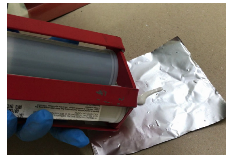
Figure 3. Dispense material to level plungers
