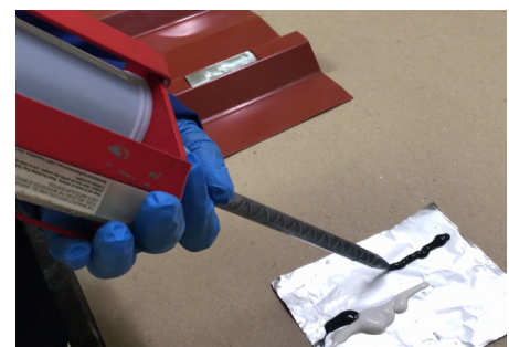
Figure 4. Attach mix tip and dispense material to ensure proper mix ratio
