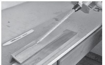
Figure 6. Position and dispense adhesive.
