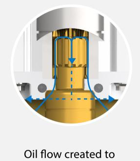
actively lubricate the spline connection
