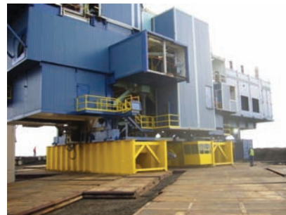
Walking system (painted yellow) uses two sets of hydraulic cylinders to lift, advance, and lower a fully-loaded rig. Each step of the walking sequence can move the load about 4 ft in 2 min.
