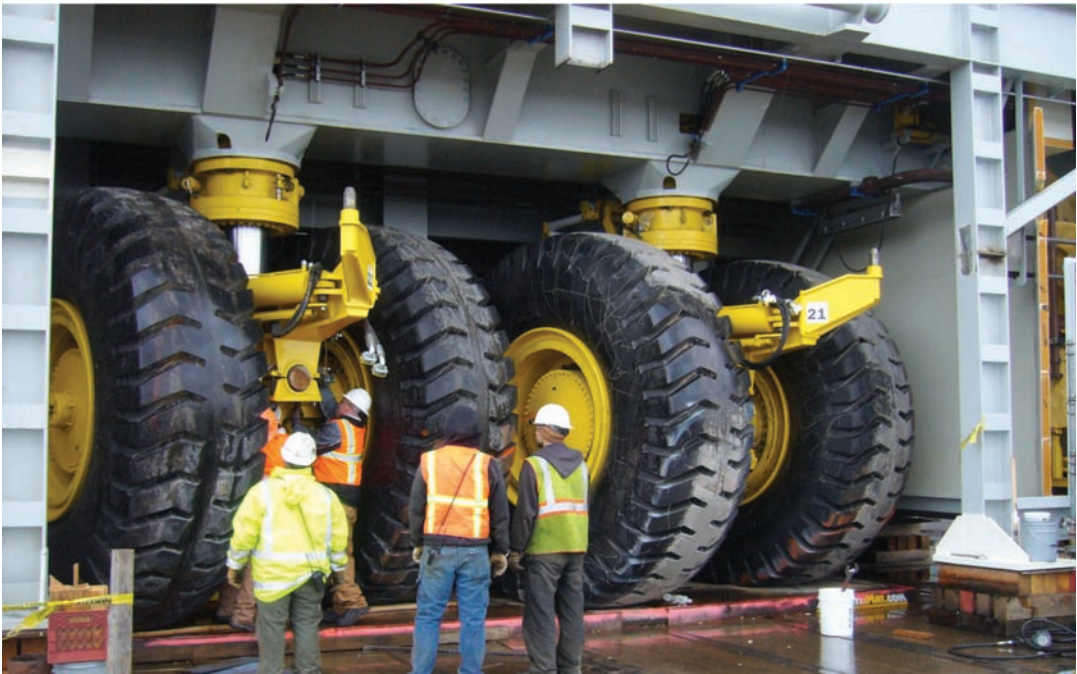
Self-propelled wheel drive modules feature a speed range of 100 ft/hr to 2½ mph and also provide hydraulic steering and braking for transporting loads to 2½ million lb.
