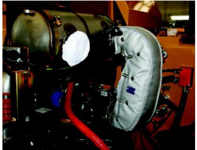
To protect the engines from damage due to water or dirt in the diesel fuel, Tigercat engineers spec'd a Racor GreenMAX fuel filter/water separator (left) for new machines. Custom-fit Firwin insulation blankets (right) help isolate hot spots in the engine compartment of this 845D feller buncher.
