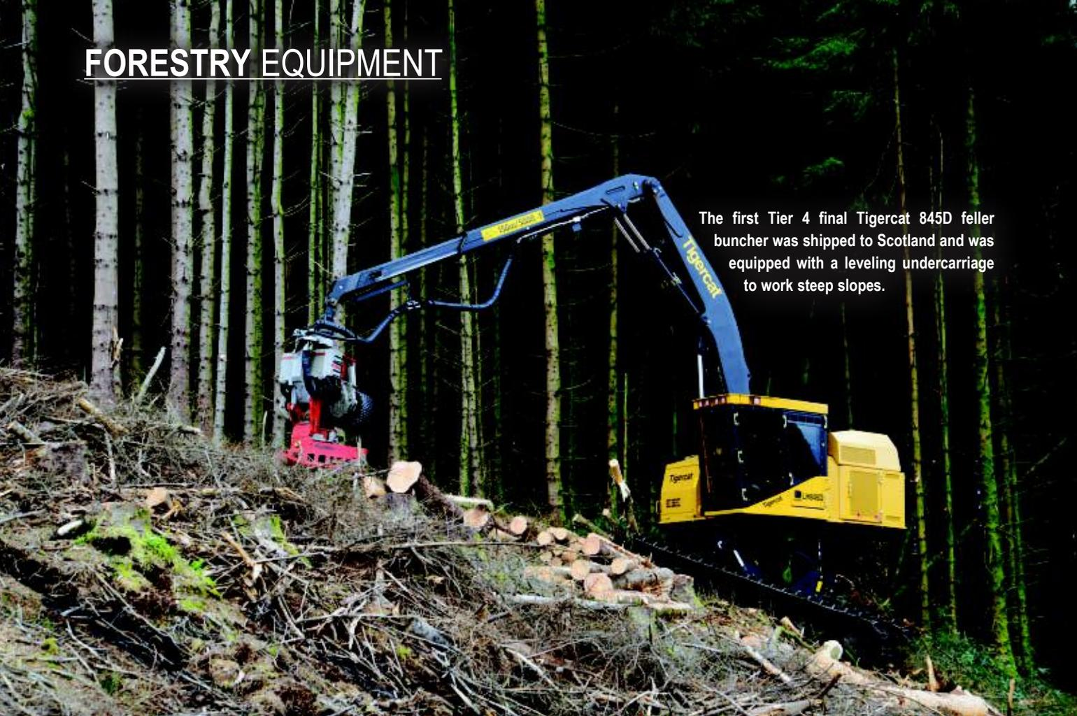
The first Tier 4 final Tigercat 845D feller buncher was shipped to Scotland and was equipped with a leveling undercarriage to work steep slopes.
