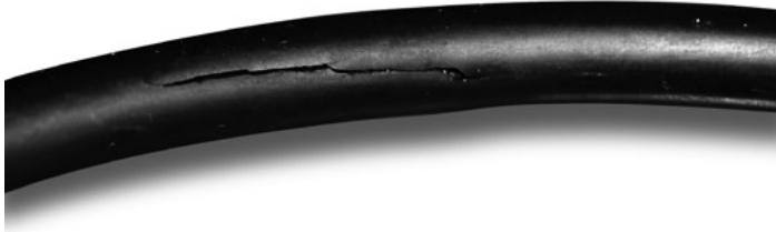
Fig. 10.11 O-Ring damaged by explosive decompression
