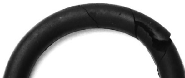
Fig. 10.10 Twisted O-Ring with cuts in surface
