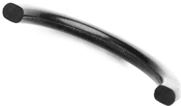
Fig. 10.8 Damage pattern caused by high compression set
