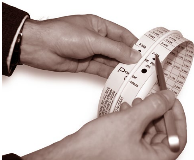
Fig. 5.5 Determination of the O-Ring size using the measuring band
