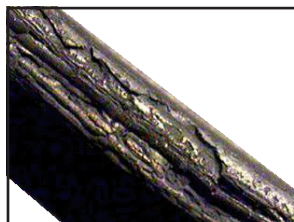
Other CR FKM Seal Seal degradation with visible cracks after <500 hours of engine test.
