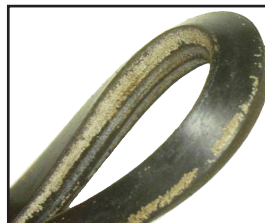
Parker's New Generation CR FKM Seal No cracks and only 9% compression set after 2000 hours of engine thermal cycle test (TCT).
