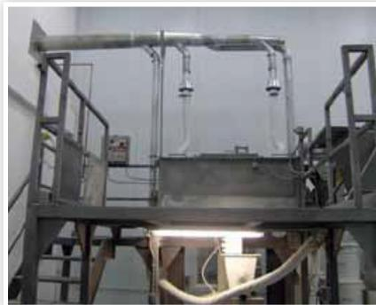
Stainless ducting is used with this dump station. Ducting is attached to DustHog SFC 32-4 above.
