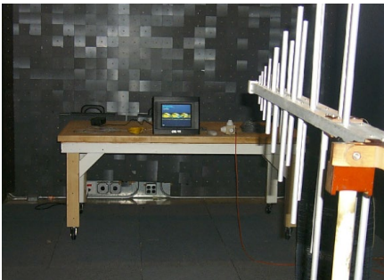
Radiated immunity test chamber (80 MHz - 2.7GHz)
