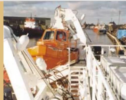
All davits supplied by VESTDAVIT are operated by hydraulic systems. In the process, the hydraulic system on board as well as the electrohydraulic device specifically designed for the task can be used.
