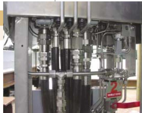
VESTDAVIT uses stainless steel O-Lok® fittings by Parker Hannifin everywhere as can be seen here in the control.
