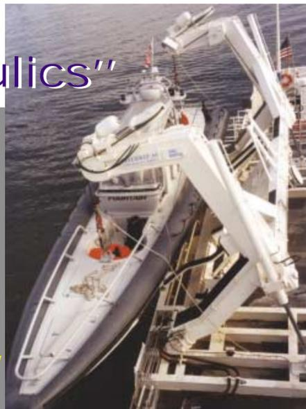
18,000 kg of hoisting capacity – that's what this davit by VESTDAVIT can handle. Its dynamic shock absorber ensures that the forces involved while the boats are launched are reduced from 1 G to just 0.2 G.
