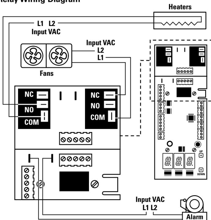
4. Connect the neutral leg of the power supply to the other lead or terminal on the fan.
