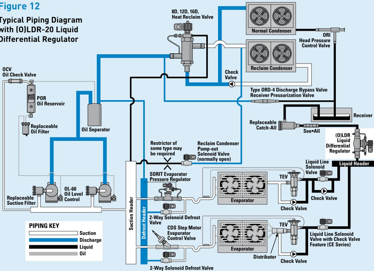
A normally open OLDLDR version or an LDR version (differential mode when the coil is de-energized) must be determined if a liquid differential pressure regulating valve is desired.
