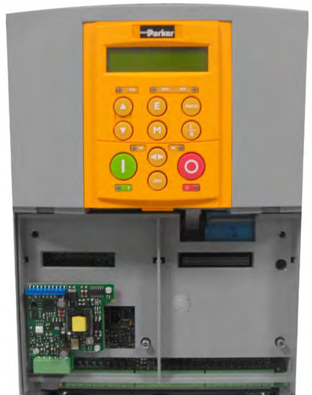
Figure 1 Encoder Receiver Option 590 Mounting
