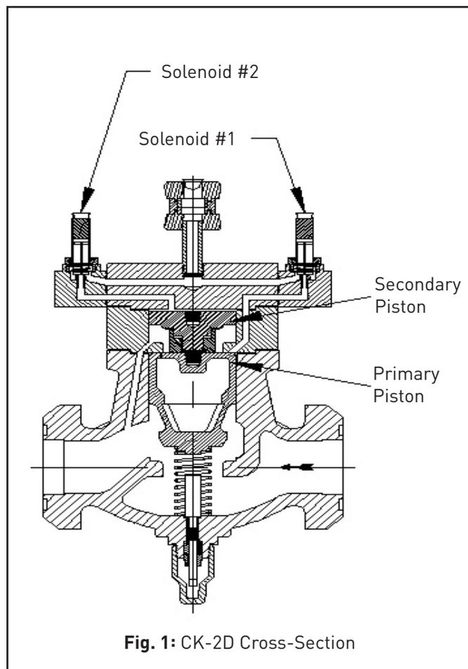
**Fig. 1: CK-2D Cross-Section**
