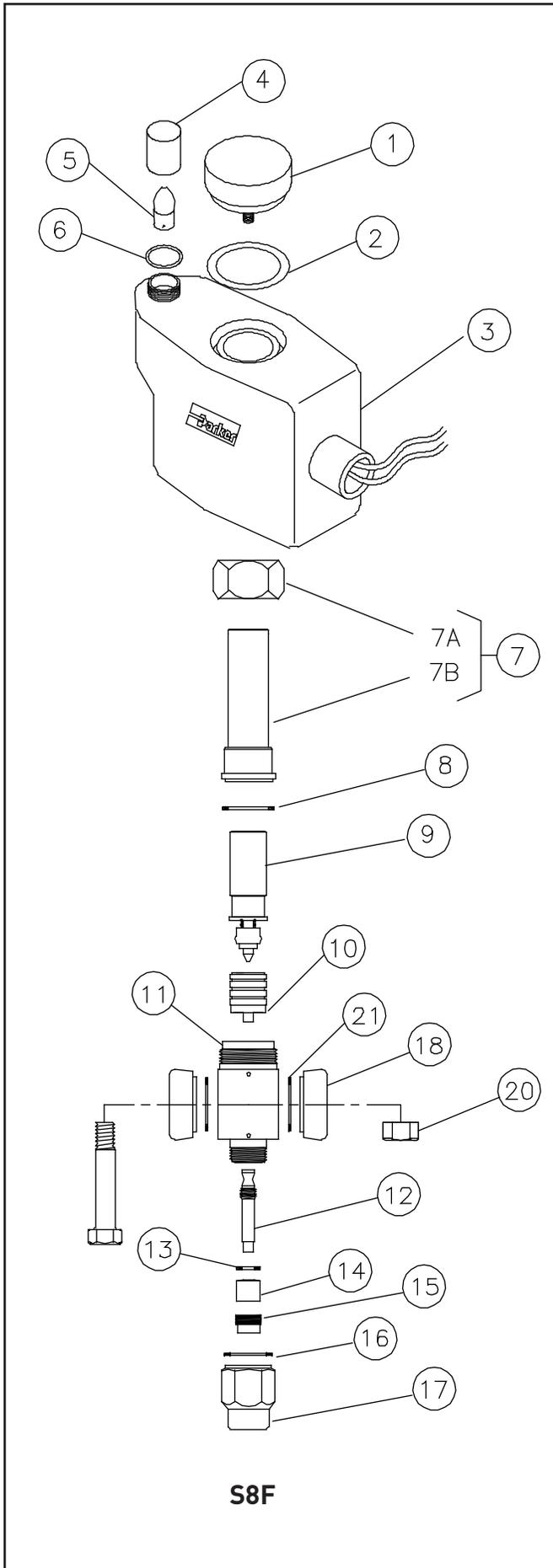
Solenoid Coil is de-energized, allowing #9 Solenoid Plunger to drop and Valve Needle to close the Pilot Port in #10 Piston Plug. Liquid and/or gas leakage through the clearance area around #10 Piston Plug causes a rapid pressure build up in Chamber A which combines with the downward force of the Spring which is part of #9 Solenoid Plunger and the weight of #10 Piston Plug Assembly to force the Main Valve Disc tight against the Seat Bead to stop all flow.
