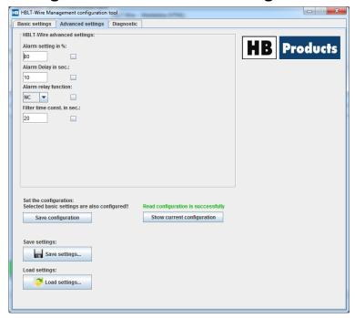
Alarm setting in %: Indicates the desired alarm level. It is given in % of max measurement range.
