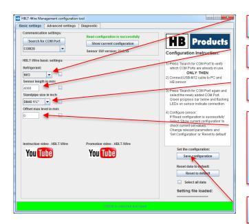
Sensor refrigerant should be input here
