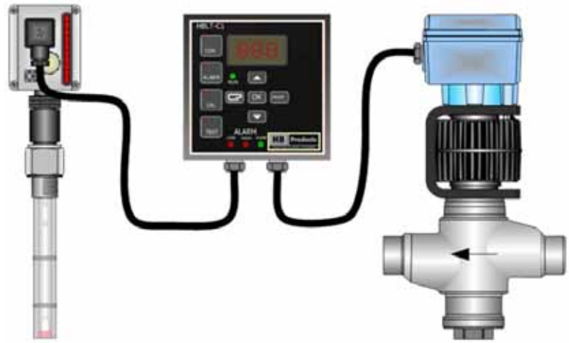
Diagram: HBLT-C1 Controller, Level Probe and MVS Motorized Valve
