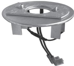
The in-filter heater is a cold weather starting aid with an internal automatic thermostat that turns the heater ON when the fuel temperature drops below 50°F (10°C) and turns OFF when the fuel reaches 80°F (27°C). Heat is supplied in the filter assembly just below the replacement filter for quick, easy starting. The 100 watt heater is operated by turning the ignition switch ON for a minimum of five minutes prior to starting the engine.
