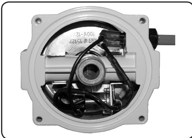
12. Now re-install the turbine centrifuge, checkball, checkball gasket, and conical parts (from step 5) onto the filter base. Start the threading process slowly so you don't cross-thread the centrifuge threads. Once started, hand tighten snugly (specification: 90 inch lbs). Double-check to make sure the heater wires are not protruding or getting pinched by the conical.
