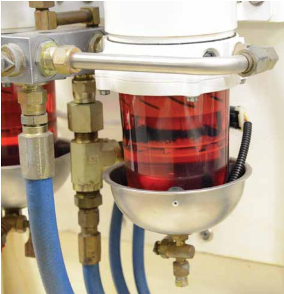
The lower section of this filter contains the centrifuge and an accumulation of asphaltene particles can be seen on the fins. The metal shield at the bottom provides a measure of protection in the event of a fire.
