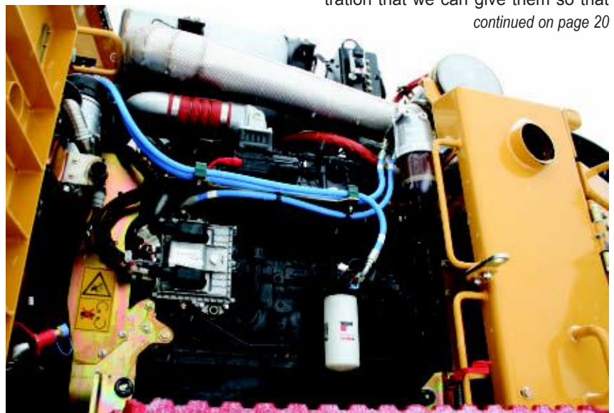
The 845D feller buncher uses a Tier 4 final FPT Industrial N67 diesel engine rated 282 hp at 2200 rpm. The red platform at the bottom of the photo is included on machines with leveling undercarriages to help make regular maintenance safer and easier.
