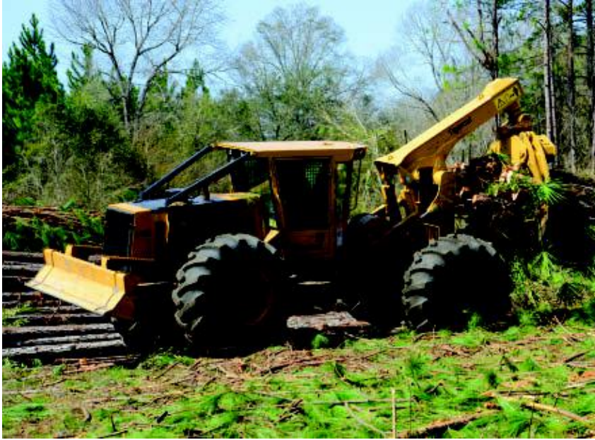
The new Tigercat 610E skidder is designed for tight spaces and soft soil conditions. It uses a 6.7 L FPT Industrial NEF N67 Tier 4 final diesel engine rated 203 hp at 2200 rpm.
