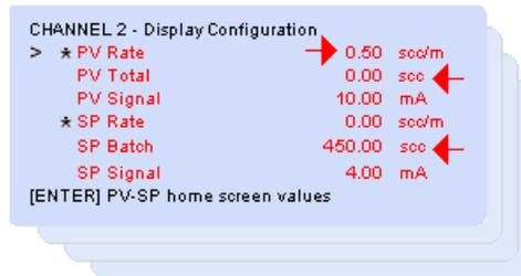
Figure 21: Image of a batch process in the display configuration screen
