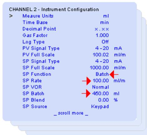
Figure 19: Image of the Instrument Configuration screen programmed in "Batch" mode
