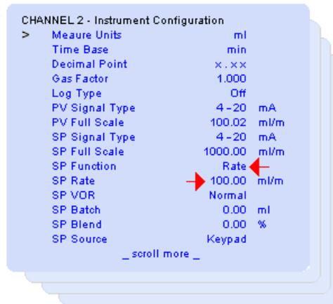
Figure 16: Image of the Instrument/ Program Configuration screen showing the SP Rate symbol
