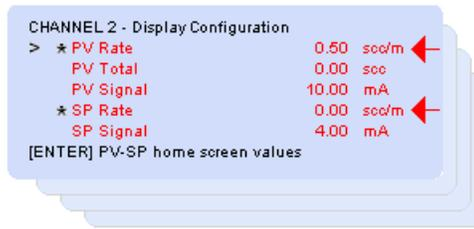
Figure 18: Image of display configuration screen showing the process is off
