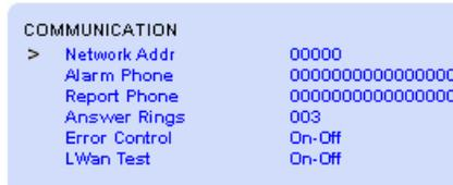
Figure 15: Image of Communications screen in Global Settings
