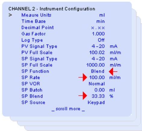
Figure 22: Image showing a blending process in the Instrument/Program Configuration Screen
