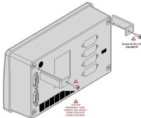
Figure 3: Panel Mount Components
