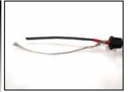
Score the inner insulation 6 inches from the end. Lightly cut the inner jacket up the center to end of heating cable and remove the inner jacket from the cable.
