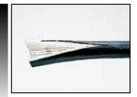
Measure 24 inches from end of bundle and carefully cut around jacket and insulation. Do not cut into heating cable or tubing.
