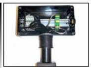
Assemble junction box to compression fitting as shown. Tighten locknut until the junction box bottoms out against the lip of the compression fitting.
