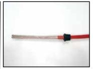
Score the outer insulation 7 inches from the end of the cable. Lightly cut the outer jacket up the center to the end of heating cable and remove the outer jacket from the cable.
