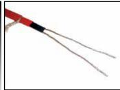
Remove the exposed core material and cut 1/4 inch of the end of each bus wire.
