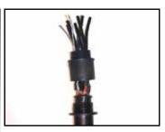
Slide compression fitting over cable. Grommet should be placed inside standoff. Termination boot should be spaced 1/2 inch from sealing grommet. Tighten compression fitting until it bottoms out against standoff.
