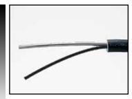
Remove jacket, insulation and heat transfer foil.
