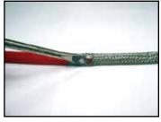
Move braid back toward the overjacket, creating a bulge. At the bulge, separate the braid to make an opening.
