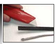
Shave the core material from the outside of each bus wire.
