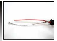
While bending the heating cable, work the cable through the braid opening. Pull the braid tight to create grounding pigtail.
